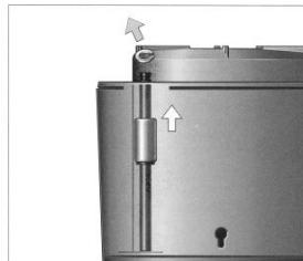
The magnetic floater is fragile. Treat with care during removal, replacement and cleaning. **The alarm contact must not be unscrewed for cleaning.** Clean the trenched plastic washer, magnetic floater, slide pipe, floater housing and alarm contact. **Remount the magnetic floater with magnet ring on the top on the slide pipe first.** Put the trenched plastic washer back on the slide pipe. Make sure that the plastic washer snaps in completely compassing the whole slot of the slide pipe.
