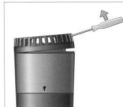
Clean with a powerful jet of water strainer, impeller and pump case. Remount the strainer on the pump case allowing it to snap in.
